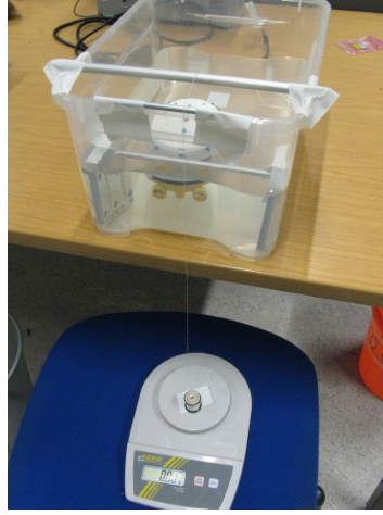
(a) Empirically measuring Lily maximum thruster force in the tank, based on its ability to lift a weight.
